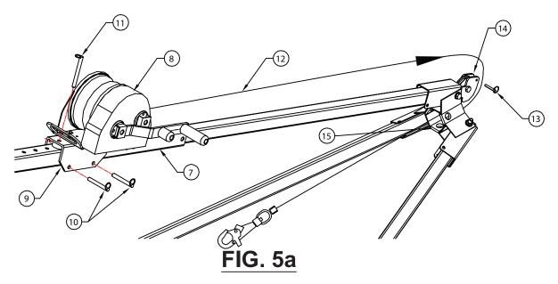
B) Installing the Winch to UCT-1000 Tripod
